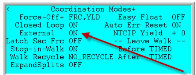
Next set up The External I/O Table (MM->2->2) to choose up to 32 patterns based on the Timing Plan Inputs and Offset input combination, that you, the user, define.
