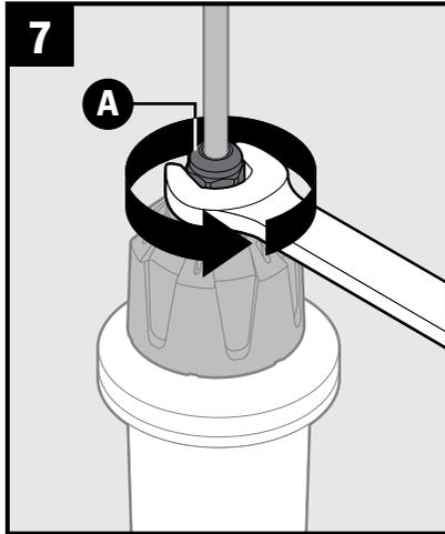
Now tighten cord grip (A), using a 3/4" wrench, to 30 in-lbs max torque.
