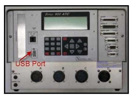
The user can backup/restore the user database to the controllers Flash Memory or to a USB 2.0 device as shown above.
