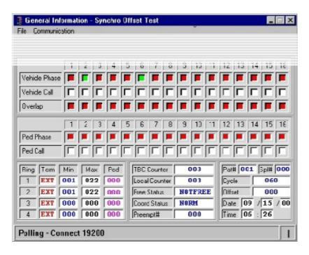
Time-base coordination uses midnight as a time reference to calculate the offset for the controller. All coordinated signal systems maintain a time-base reference by zeroing the cycle counter at midnight and accumulating cycle times to the current time. You can confirm this for the examples covered so far because
