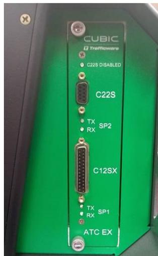
ATC Cabinet Card must be plugged in before COMMANDER is powered up.
