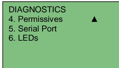
NOTE: Diagnostics can be disruptive and are meant to be used for production testing. Latching and Logging of the test results can be controlled through the Diagnostic latch in the configuration menu under latching.
