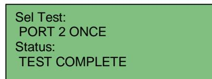
To execute the self-test, install the loopback connector on the port to be tested. Then select the port and test to be run below the prompt "Sel Test:". The status will be displayed during the test and the results when it is complete. If "PORT 2 CONT" is selected, the test will be run continuously. In this case, a successful test is one that continues to display a status of "RUNNING". If the "PORT 2 ONCE" test is selected, a successful test displays "TEST COMPLETE". An
